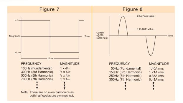
The only useful current is the fundamental component of current, as it is only this that can generate useful power. The additional harmonic current not only flows within the power supply itself, but in all of the distribution cables, transformers and switchgear associated with the power supply and will thus cause additional loss.
