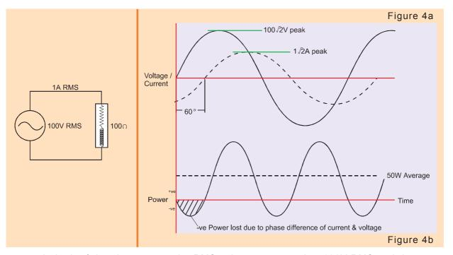
In both of the above cases the RMS voltage was equal to 100V RMS and the current was 1A RMS. The product of these two values is the apparent power delivered into the load and is measured in VA as follows:
