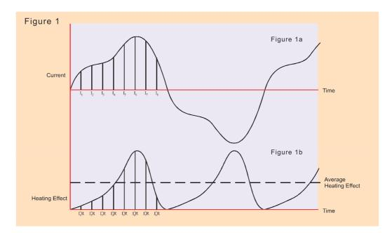
If this current is considered to be flowing through a resistance, the heating effect at any instant is given by the equation:
